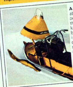
A serviceman's dream. No doubt about it, SKI-DOO for '68 is the pest performing snowmobile on the market . . . and designed to keep it that way! Everything has been engineered for simplest tuning, fastest servicing. The entire cabin is held down by four, easily removed, winged lockruts. A new cylinder head makes it easier to change spark plugs. Decompression switch is easy to remove for engine servicing. A new pulley and drive belt guard can be removed and replaced in a jiffy.
