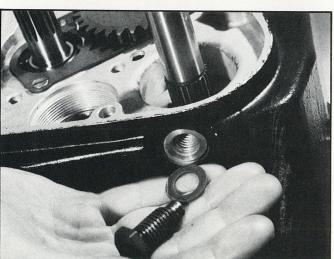
Remove the kick starter stop bolt and its sealing
