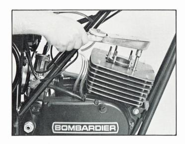
Replace the cylinder head and tighten cylinder head nuts gradually, to the specified torque, using a criss-cross sequence.
