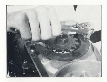
Remove the three (3) bolts and locking washers securing the chain guard.
