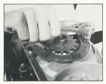
Fit the chain guard with its 3 distance spacers. Secure it with 3 bolts and lock washers.
