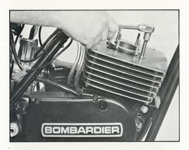
13. Gradually, and in a criss-cross sequence, torque cylinder base nuts to 20 ft/lbs. (2.8 k.p.m.).
