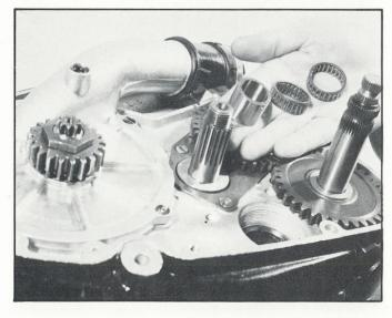
Remove the two (2) clutch drum bearings and the inner bearing race sleeve.
