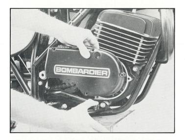
Remove the four (4) Allen screws retaining the magneto cover. Remove the magneto cover.
