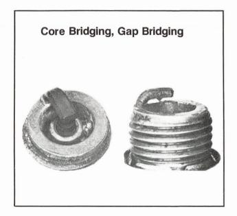
Combustion particles wedged or fused between the electrodes or the core nose and shell.
