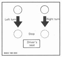
To steer the vehicle in a given direction, pull the lever corresponding to that direction.
