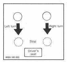
Steering is effected by means of the steering levers, through the planetary-type controlled differential. Pulling on one lever applies the brake on one drum of the differential. This slows down the axle gear of that side and increases proportionately the speed of the axle gear on the other side. One track running faster than the other makes the vehicle turn. With this type of differential, there is traction on both tracks, even when turning.
