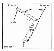
This brake works with a disc. Brake tension can be adjusted by turning the handle in one direction or the other. Turn clockwise to increase tension and counterclockwise to reduce it.
