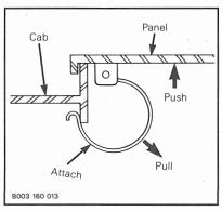
To open, pull on both retaining locks and push the panel.
