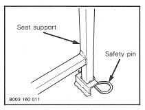
To gain access to the batteries remove the safety pin and tilt the driver's seat towards front.
