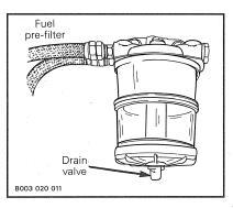
To drain the water accumulated in the pre-filter, open the drain valve slowly and let the water come out. When fuel starts flowing, close the drain valve.
